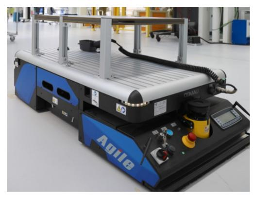
Tracking AGVs as they displace items from the warehouse to the workfloor
